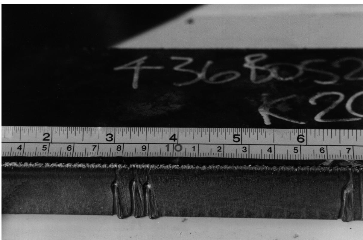
Figure 4 Unacceptable isolated defects in flame cut surface
