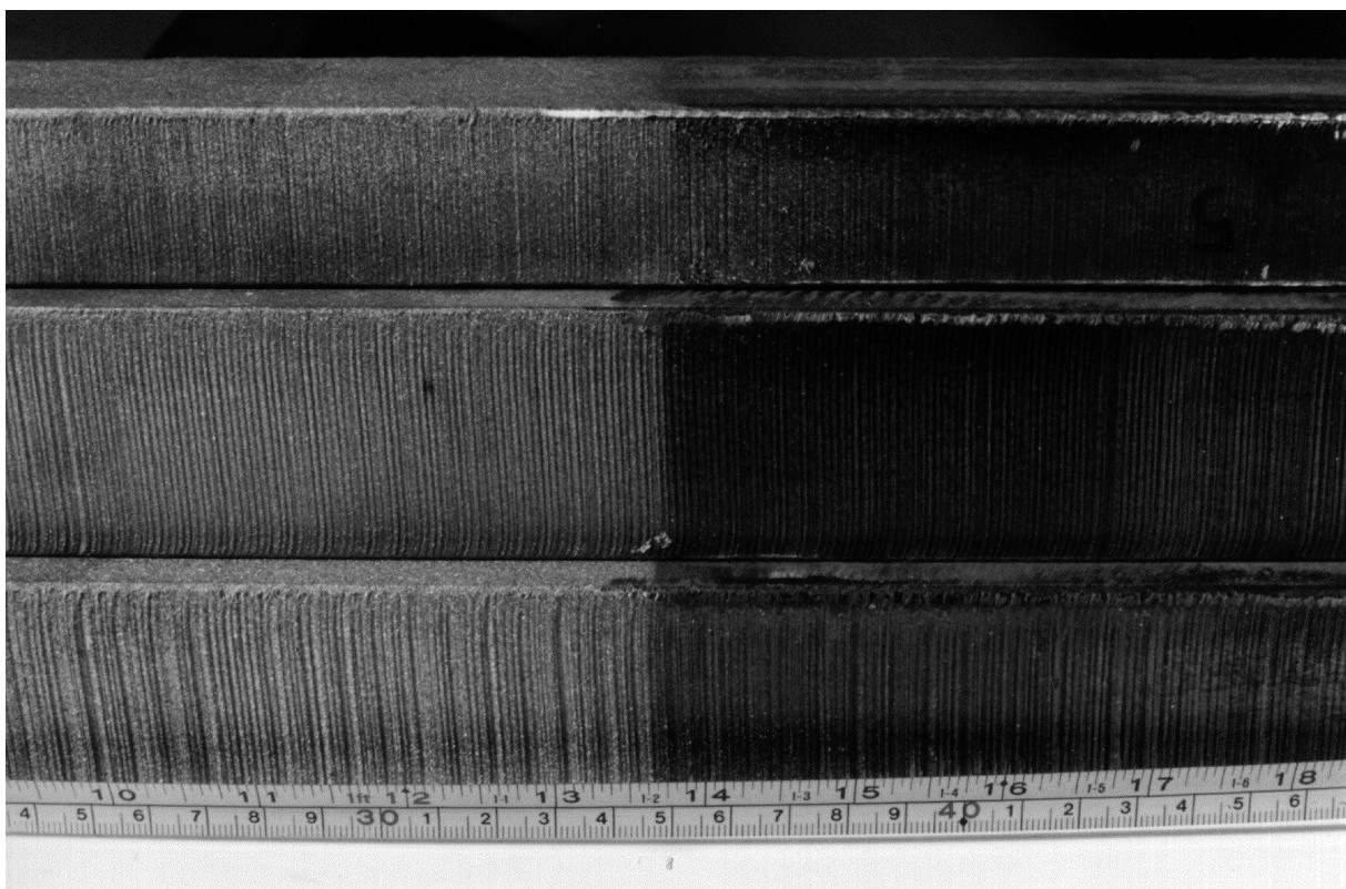
Figure 3 Drag lines produced by flame cutting
