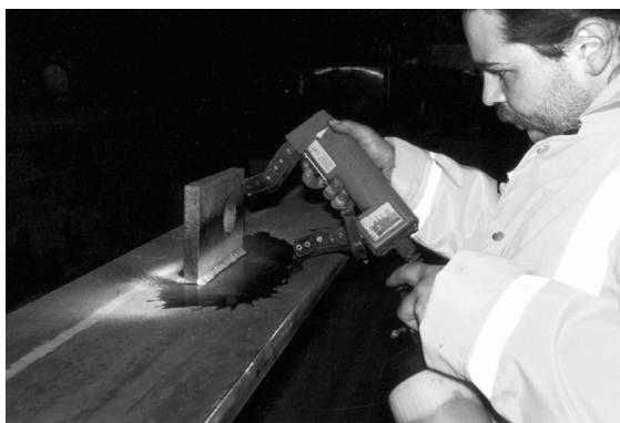
Figure 1 Setup for MPI
