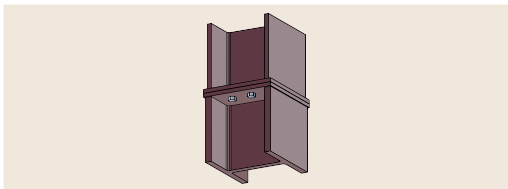
Figure 7.7 Cap and base column splice
