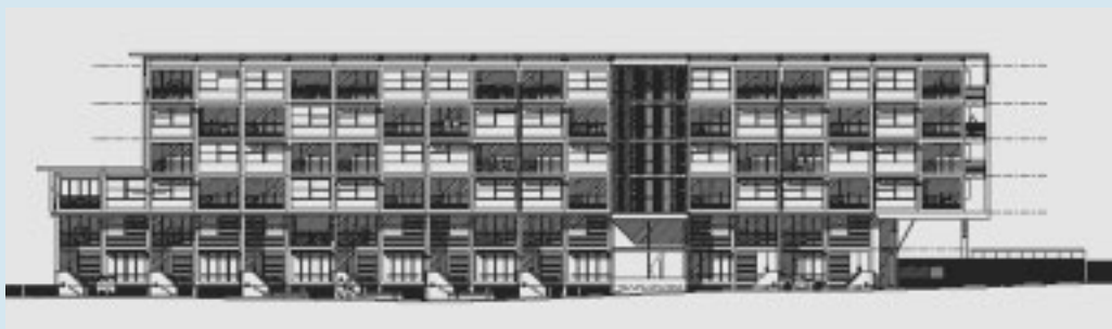
Representation of building showing the set-back and overhangs at second floor level
