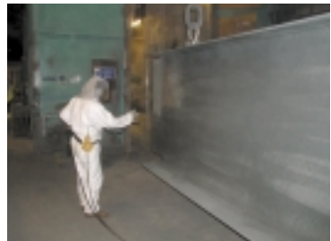
Shop applied protective treatment
