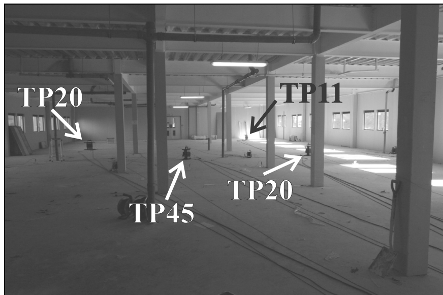
Figure C.5 Multi-shaker modal testing setup.
