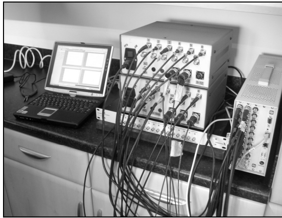
Figure C.4 Typical PC-based data acquisition setup.
