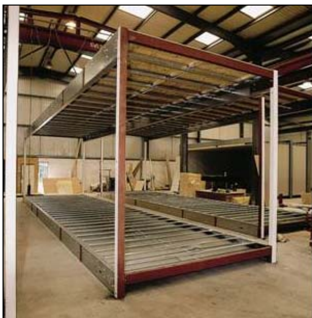
Figure 11 Primary steel frame used in an open-sided module Courtesy, Kingspan Off-Site and Modular UK
