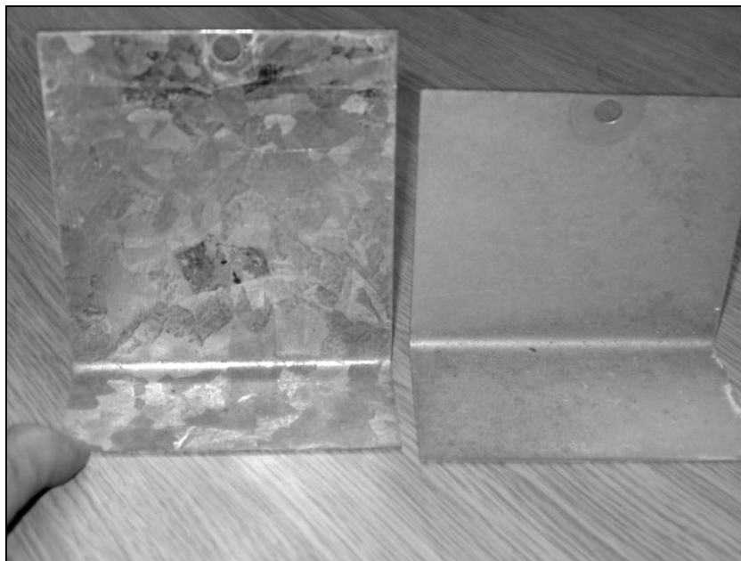
Figure 3.11 Chromated and non-chromated zinc coupons after 13 years exposure (non-chromated zinc coupon on right)
