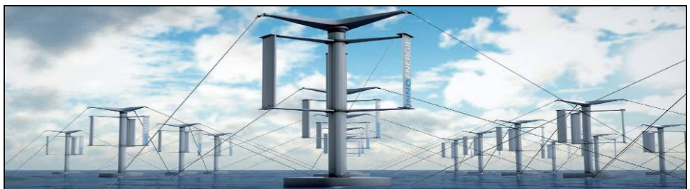
Figure 5.17 Array of small-scale vertical axis wind turbines on a flat roof
