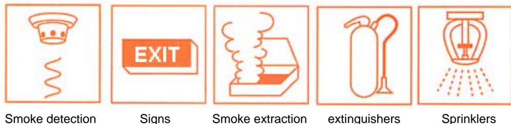
Figure 6.4 Active fire protection methods
