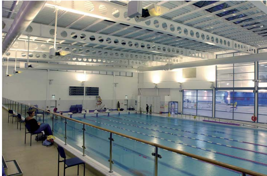
Figure 3.15 Beams with circular web openings
