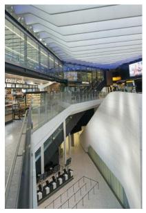
By taking a fire engineering approach and limiting the fire load within the passenger concourses, it was possible to omit fire protection to the exposed steelwork.
