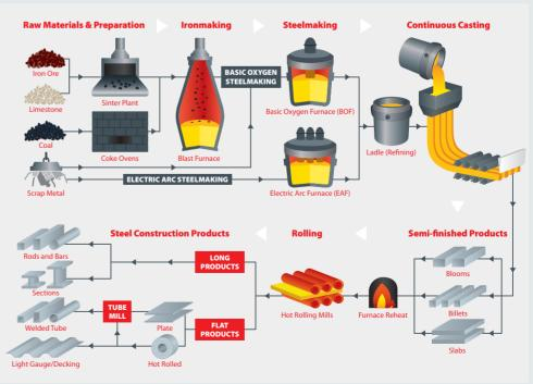
» (BF-BOF) and the 100% scrap-based steelmaking process using an electric arc furnace (EAF) together comprise a single global system of supply to meet the increasing worldwide demand.
