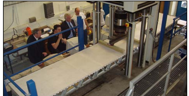
Structural tests on lattice joists at the University of Surrey
