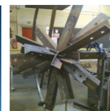
Development of one of the 547 nodes, which bring together up to 29 steel members.
