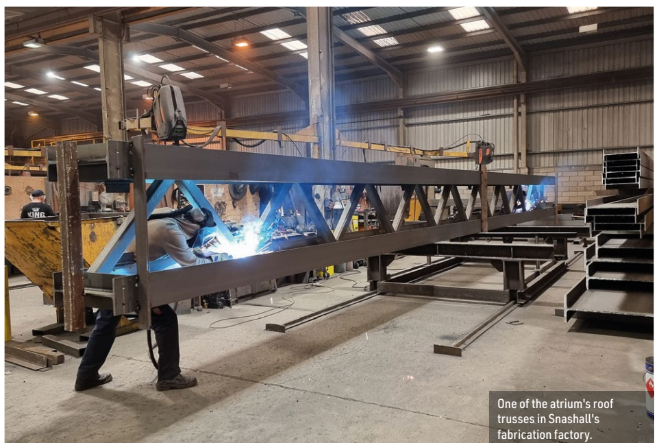
Four trusses span the atrium and support rooflights.
