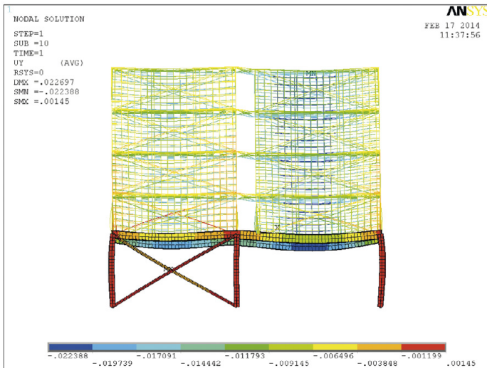
(a) Deflection (exaggerated) of steel frame supporting modules
