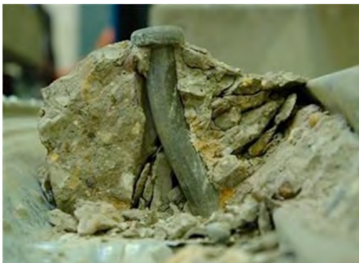
Figure 5.5 Local failure of the concrete surrounding a shear stud in trapezoidal decking
