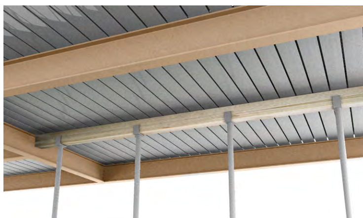
Figure 4.18 Temporary support using 'Acrow' props
