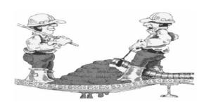
The maximum deviation is only +20mm. Do not pour to the datum as a constant thickness is required across the decking surface.
