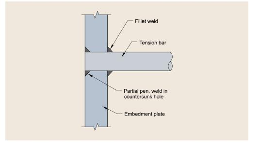
Figure 6.1 Suggested weld detail – cast-in plate to reinforcement
