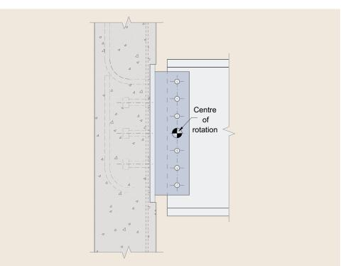
Figure 2.2 Centre of rotation of joint
