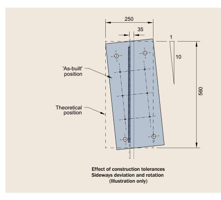
Figure 5.2 Construction tolerances
